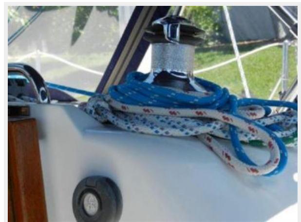
Electric Winch on cabin top
