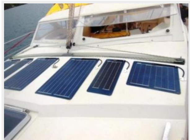
solar panels on deck
