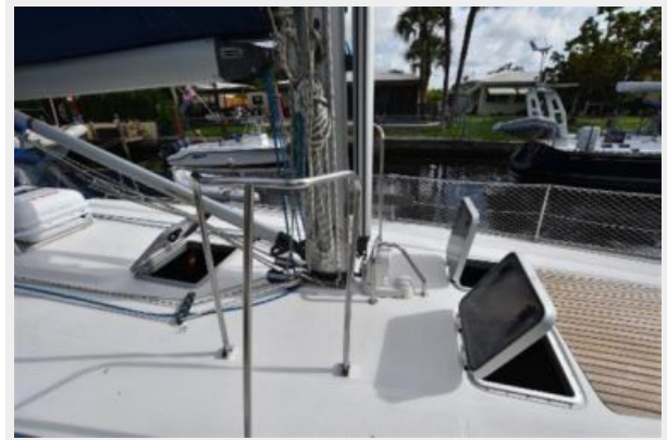
Mast pulpit for safety
