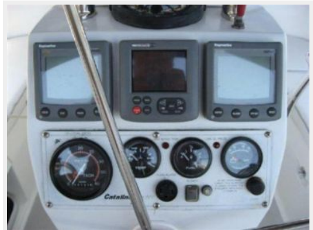
Engine panel and ST 60+ Depth and Speed and ST 70 autopilot
