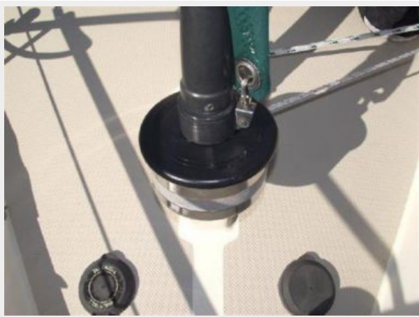
Roller furling/windlass controls
