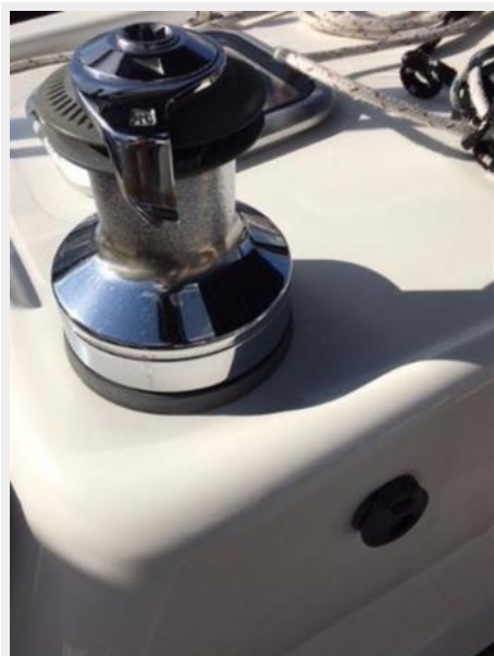
Electric maneuvering winch, port side deck house
