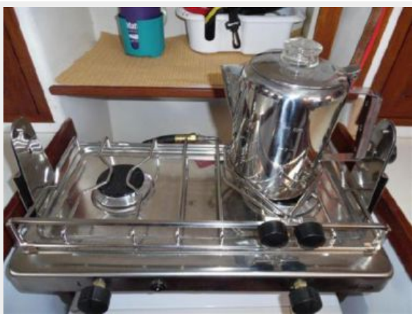
New Propane Stove (Gimble)
