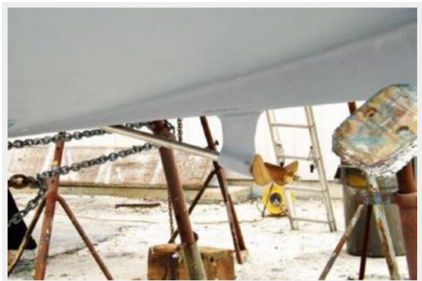
New Barrier Coat and New SS Shaft
