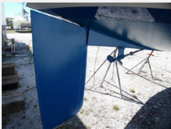
New Bottom Paint, No Blisters
