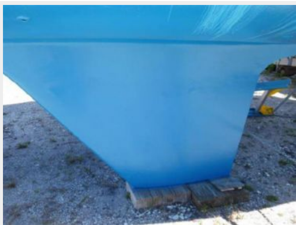
New Bottom Paint, No Blisters
