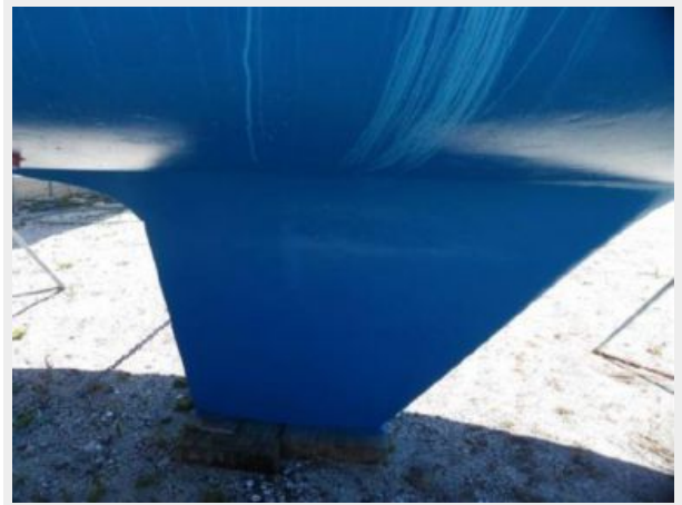
New Bottom Paint, No Blisters
