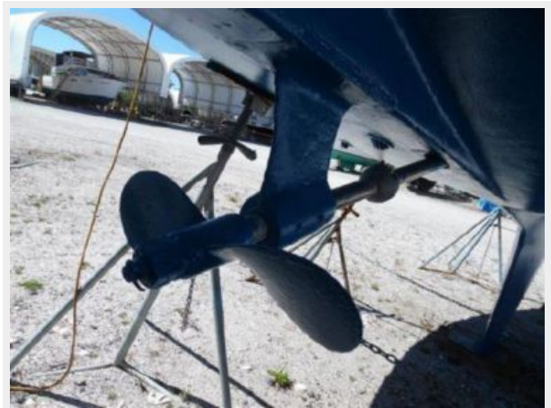
New Bottom Paint, No Blisters
