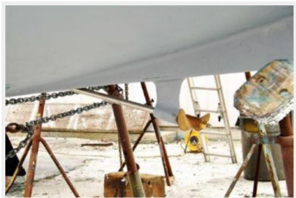
New Barrier Coat and New SS Shaft
