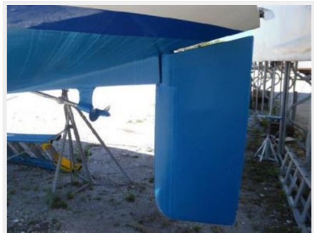
New Bottom Paint, No Blisters
