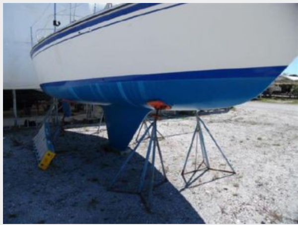
New Bottom Paint, No Blisters
