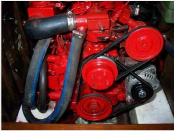
Westerbeke 12B Diesel Engine Under Stairs
