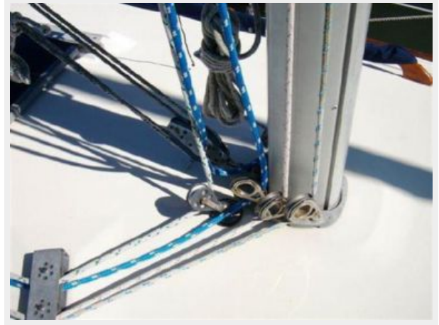
Mast Base_Lines Led Aft
