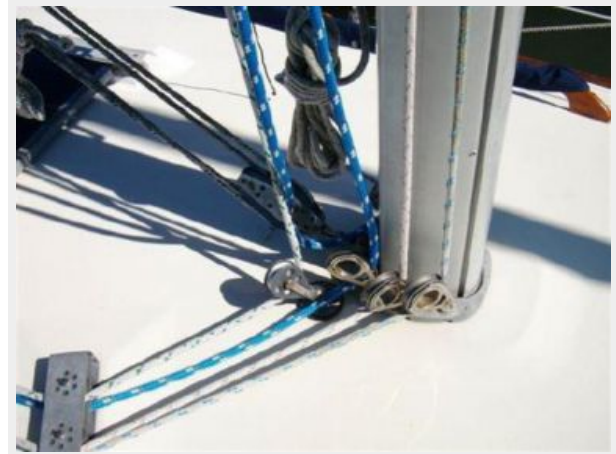
Mast Base_Lines Led Aft
