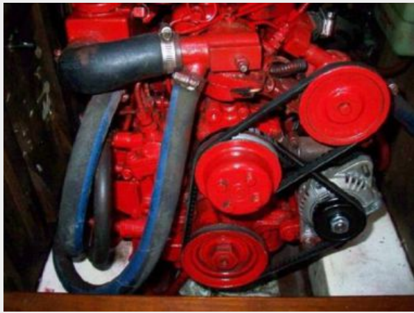
Westerbeke 12B Diesel Engine Under Stairs
