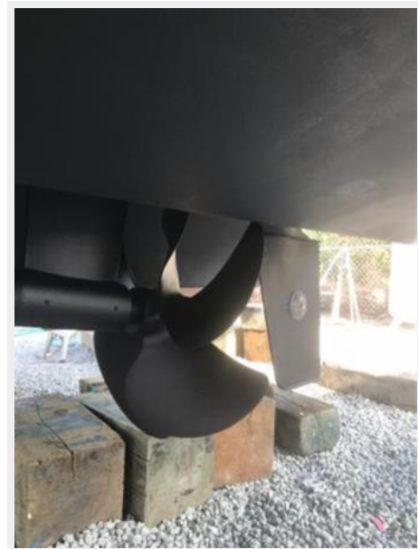
Charisma - Port propeller, rudder, shaft, and struts with fresh bottom paint (March 2018)
