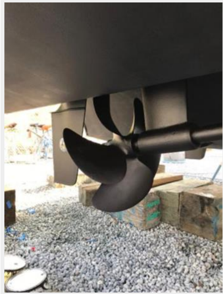
Charisma - Starboard propeller, rudder, shaft, and struts with fresh bottom paint (March 2018)
