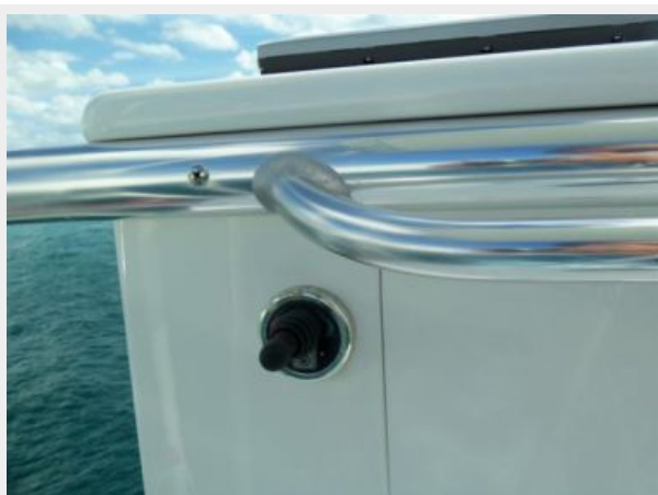
Tower Thruster Control
