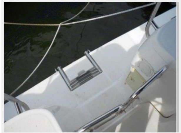
Swim platform and ladder. Note the grab rails on either side.
