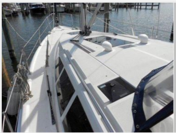
The coachroof is clean and uncluttered. Note the inboard shrouds for higher sheeting angles
