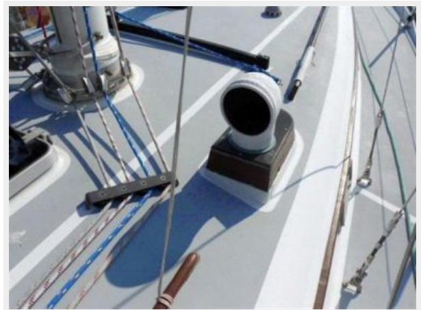
Lines are led aft to the cockpit
