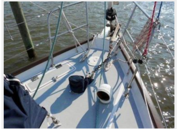
Foredeck with double bow rollers. Note the dedicated Danforth locker on port
