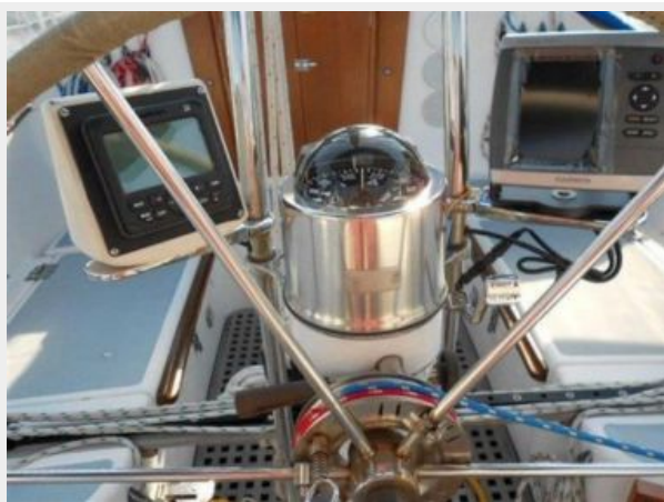
Simrad autopilot, Garmin chart plotter and a Monitor windvane
