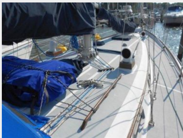
Looking forward; note the self-tending staysail
