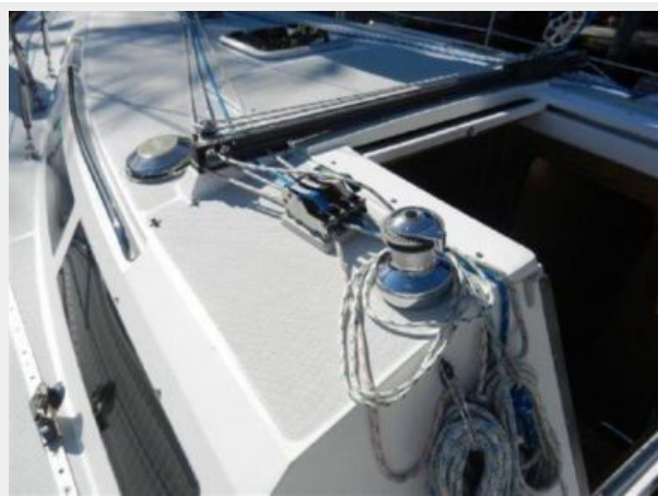
All lines led aft, Port Side
