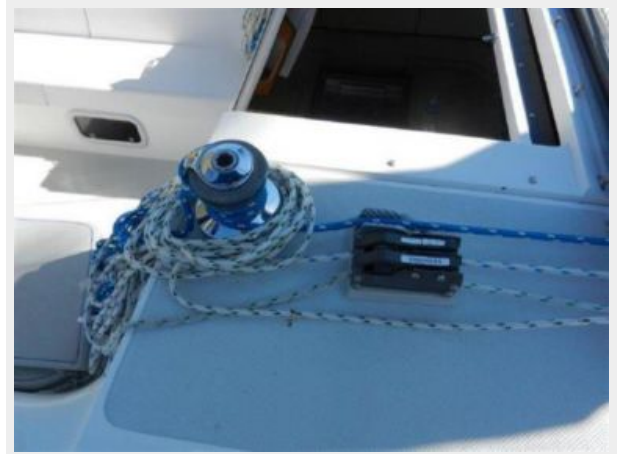
All lines led aft, Starboard Side
