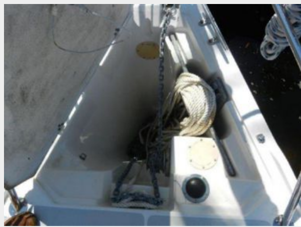
Clean anchor locker with windlass
