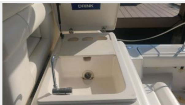
Wet Bar Sink
