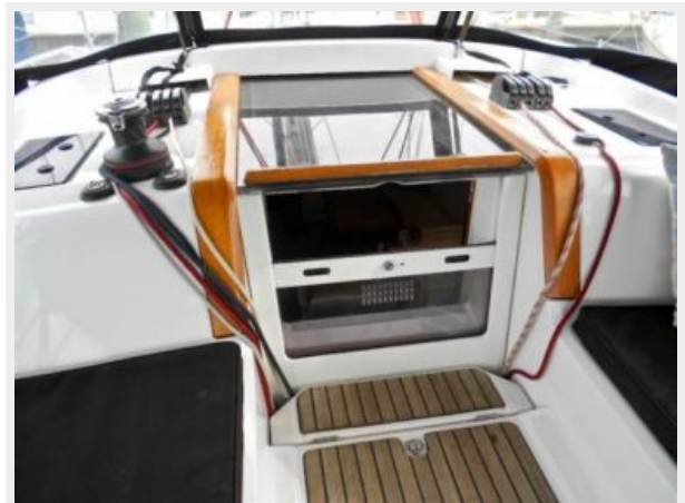
Line tails stow away beneath the self-stowing companionway boards
