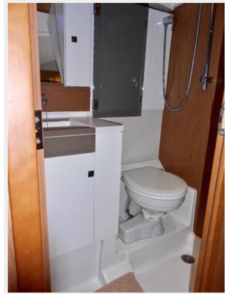
Fresh water flush electric heads
