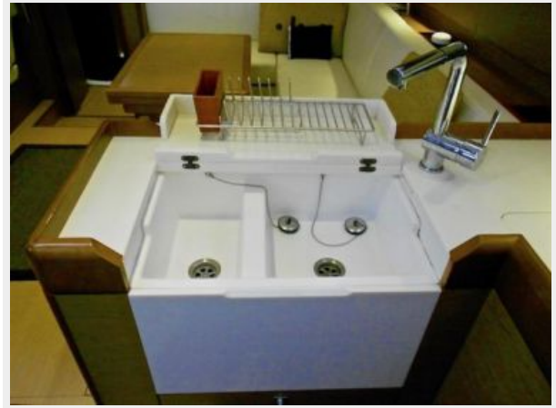
The sink cover folds and slides back to open up the sinks and provide a place for sponges and soap while you wash
