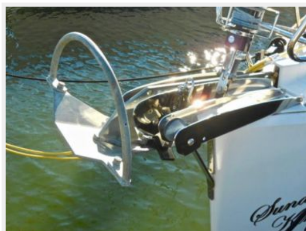
The windlass is mounted below deck as well A beefy Mantus anchor and all chain rode
