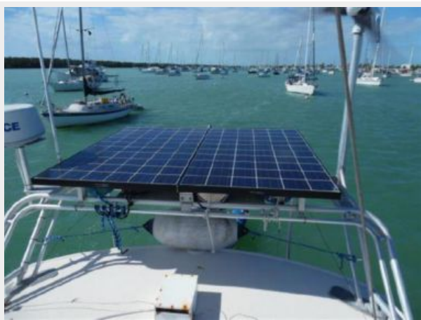
2 - 15 Amp Solar Panels
