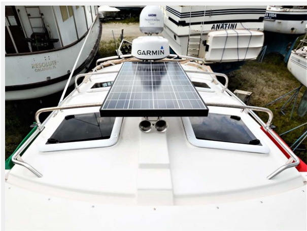
Solar Panel and Radar
