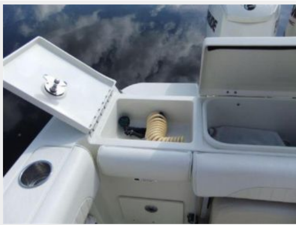
Transom wash down compartment
