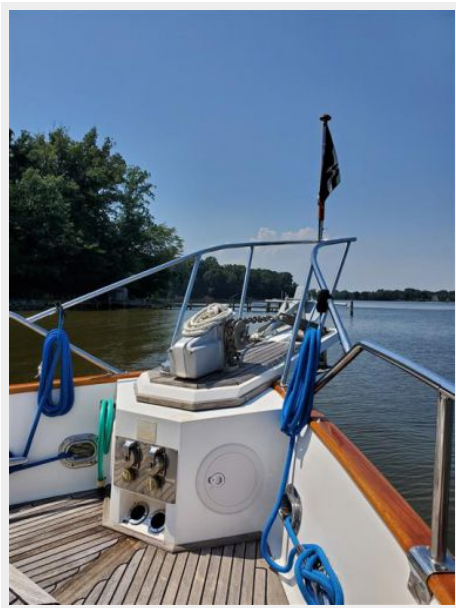
Foredeck with anchor windlass and anchor platform, teak deck
