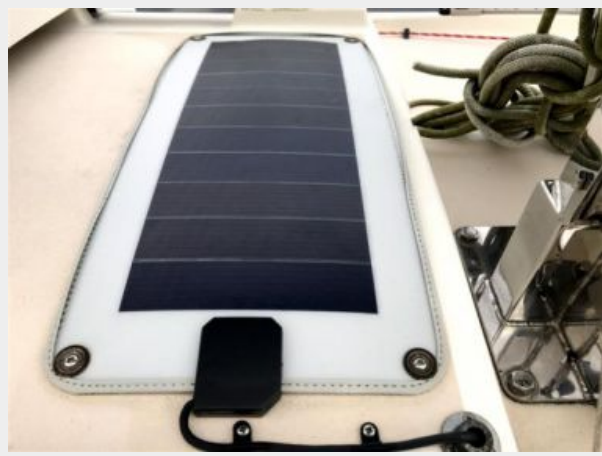
solar house bank charger
