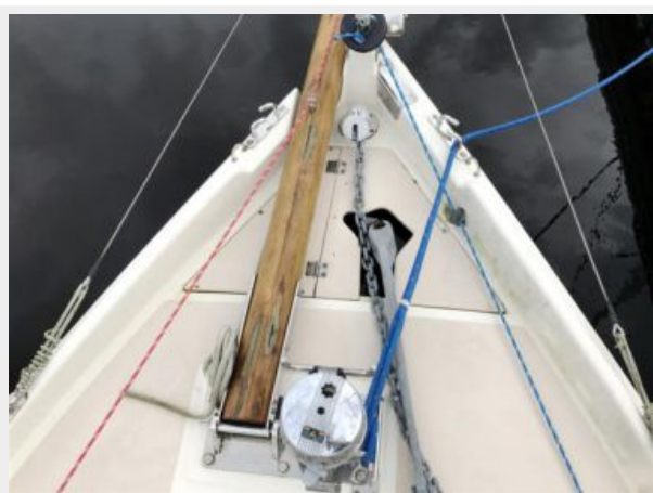
anchor locker and windlass
