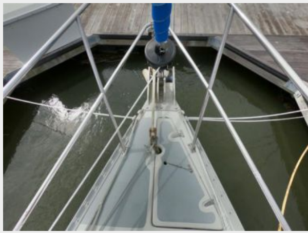
roller furling jib and anchor locker
