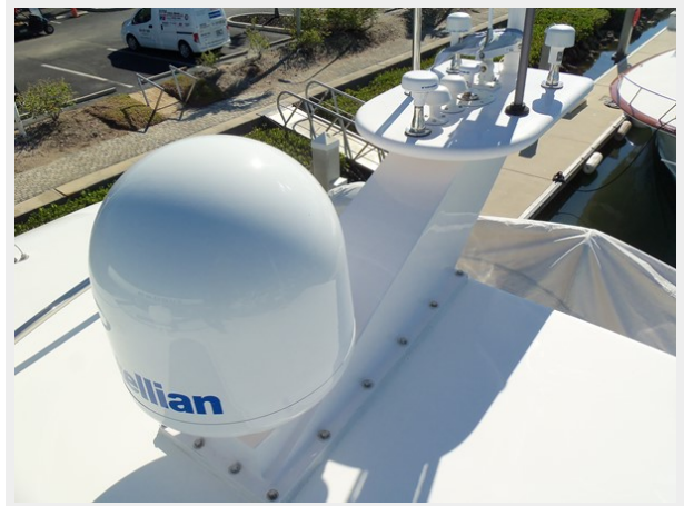
Coach Roof Mast
