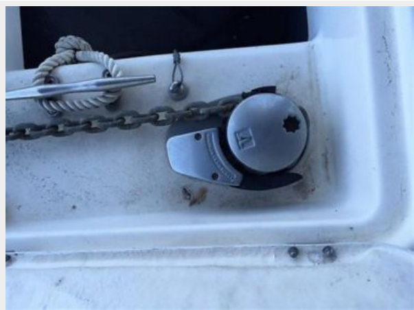
4.3 The Blessing 2000 Silverton 352 Windlass
