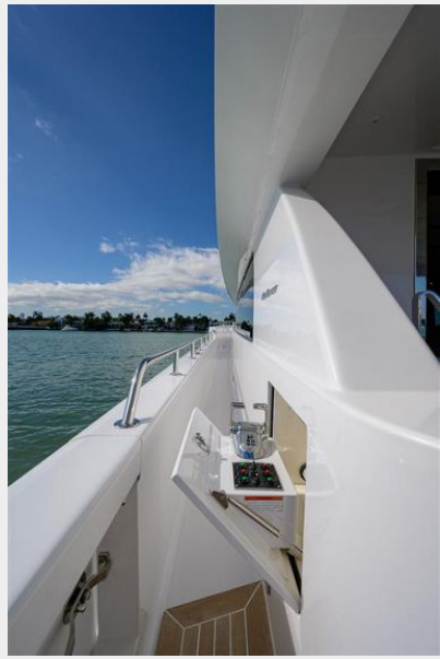
Aft Deck Control Station Port Side
