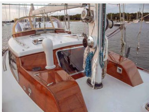
Mast Base / Coach Roof
