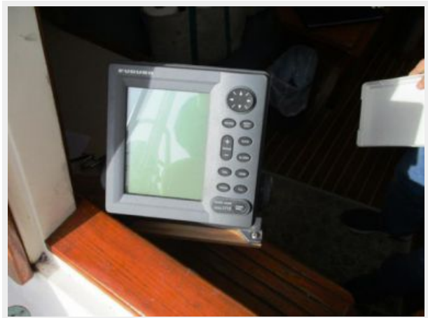
Companionway custom radar bracket
