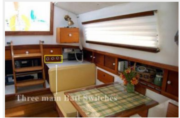
14 Pippin Batt Switches
