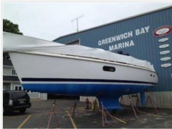
Topsides and bottom freshly painted
