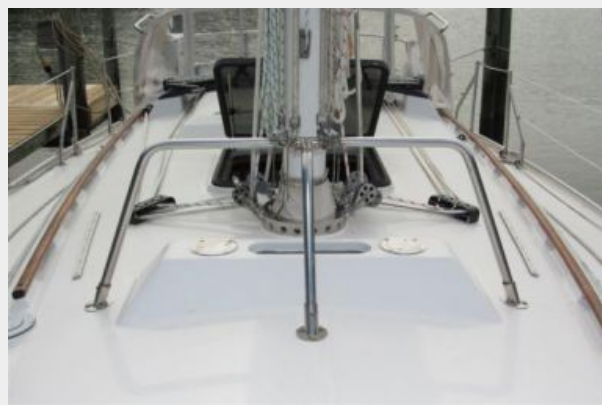
S/S guard at mast
