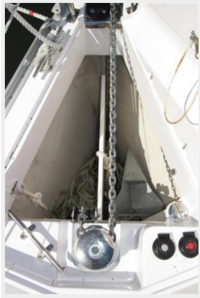
Anchor locker and windlass
