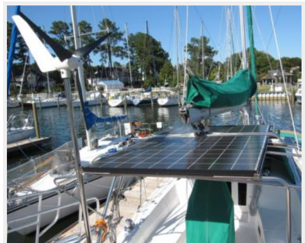
Solar panel & wind generator
