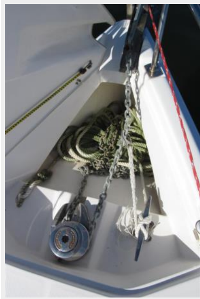
Anchor locker and electric windlass
