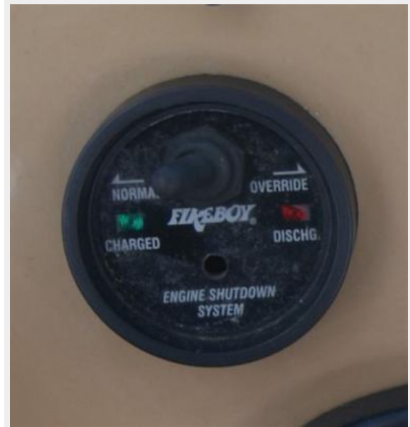
311 FireBoy Engine Shutdown
