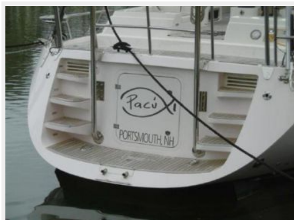
Sugar scoop transom with access to watertight storage compartment
