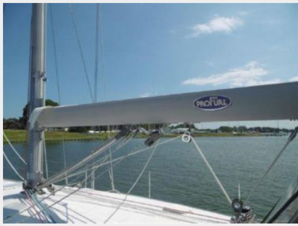
Upgraded ProFurl inboom mainsail for better sail shape
