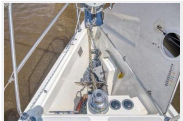
Chain locker and refurbished windlass
