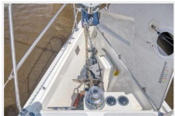
Chain locker and refurbished windlass
