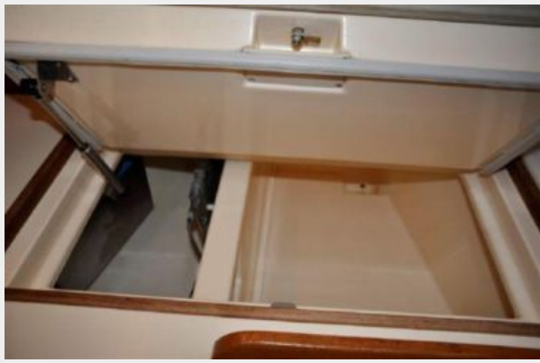
icebox with divider and plate freezer units and spillover fan
