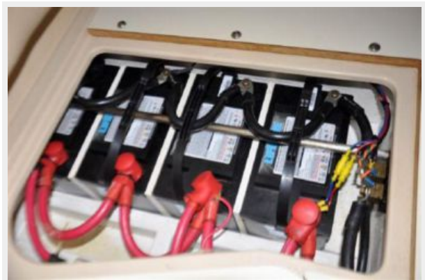
Four 100 amp/hour gel cells for the house
