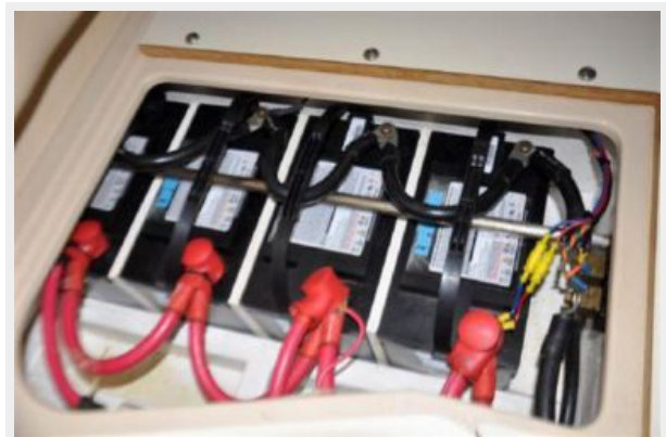
Four 100 amp/hour gel cells for the house
