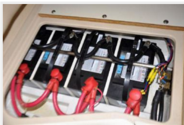
Four 100 amp/hour gel cells for the house
