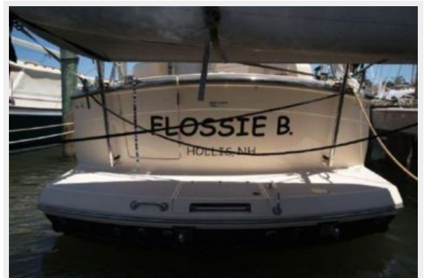
Swing platform and transom door
