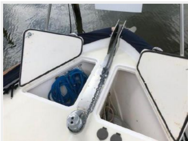
Anchor Well, Windlass
