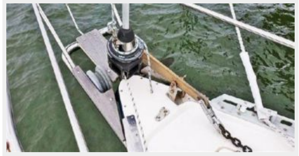
Dual Roller Anchor Platform
