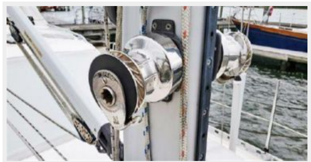
Anderson Mast Winches
