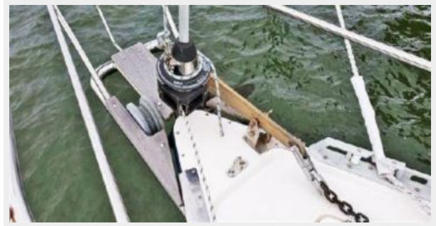
Dual Roller Anchor Platform
